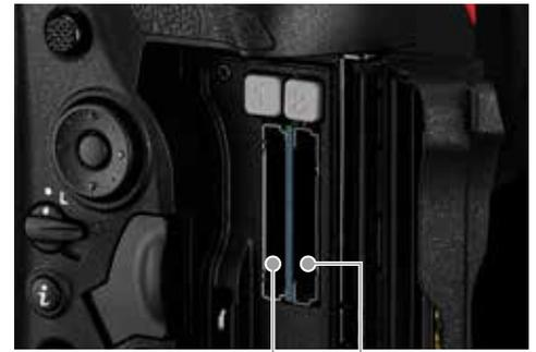
**Slot 1:** JPEGs recorded in size and quality set using the Qual button or still image recording menu
